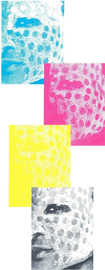
Above, an image separated into the four process colors.
