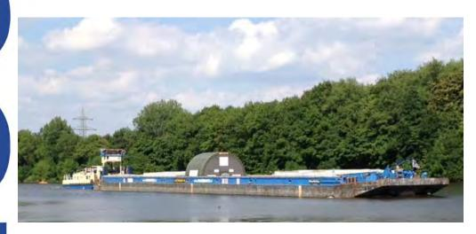
Yankee cylinder being transported to the mill
