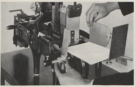
ELLIOTT MODEL "125" OPERATION No. 2 Here the operator is setting the side and end guides to correspond with the exact *size* of the envelope. Note in this demonstration the medium size of Warren's Standard Booklet Envelopes used
