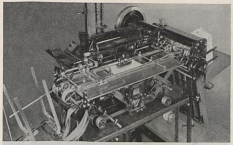
ADDRESSOGRAPH MODEL "A-4" OPERATION No. 3 The envelope is now in printing position. Notice how the flaps all are outside the printing area, thus providing a perfectly even printing surface for the address. This feature of Warren's Standard Booklet Envelope makes for better and clearer addresses
