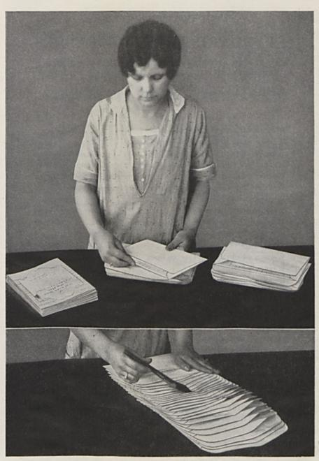
INSERTING (Top Illustration) OPERATION No. 4 After pushing the booklet firmly into the envelope, arrange them with flap open in a pile convenient to handle
