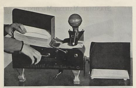
STANDARD MODEL "G" OPERATION No. 3 The gummed envelope flap is shown riding smoothly over the moisture slot. The scientifically designed curve of the flap assures a new degree of smoothness and speed in this important part of the process
