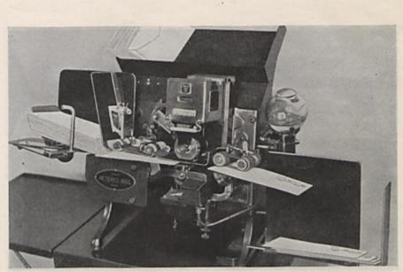
PITNEY-BOWES MODEL "B" As it passes through the pressure rolls, the flap of the Warren's Standard Booklet Envelope is securely and rapidly sealed. Note the next envelope smoothly approaching printing position
