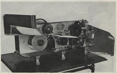
STANDARD POSTAL PERMIT PRINTER AND SEALER OPERATION No. 2 The first envelope is in position for printing the indicia on the front upper right corner of the envelope. Note the printing plate directly over the front corner of the envelope
