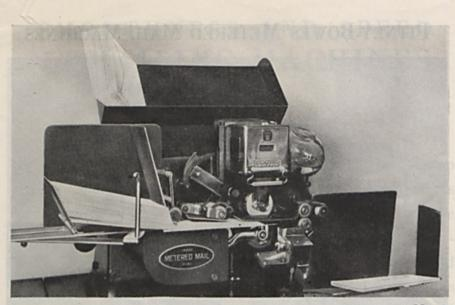
PITNEY-BOWES MODEL "B" The bottom envelope, pushed along by the feeder roll, has run smoothly into position for printing the metered mail indicia in the usual corner
