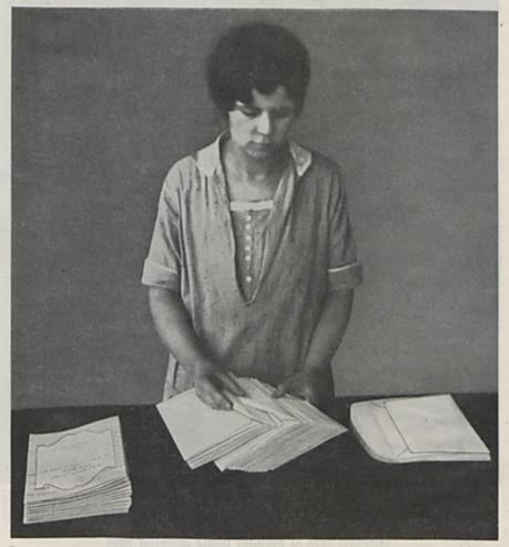
INSERTING OPERATION No. 1 The first time and labor saving operation is to open the flap and pile the envelopes with the flap side up ready for inserting
