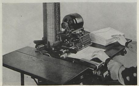
ADDRESSOGRAPH MODEL "F-2" OPERATION No. 1 The operator is inserting the envelope in this hand fed Addressograph. The envelopes are inserted flap up. Note again how the arrangement of end and top flaps provides ample even space for addressing
