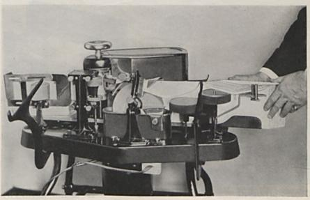
PITNEY-BOWES MODEL "AM" OPERATION No. 4 Rear view of the MAIL-O-METER showing the start of the sealing process. The envelope flap is passing across the cone shaped moistener, the curve of the flap meeting the curve of the moistener smoothly and swiftly
