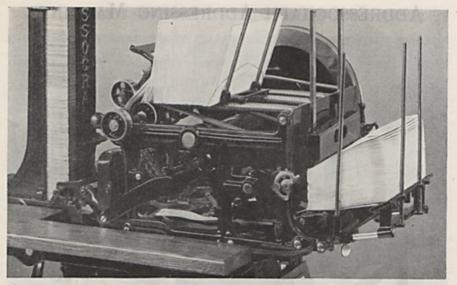
ADDRESSOGRAPH MODEL "A-1" OPERATION No. 3 An all-operation view showing how smoothly these large sizes of Warren's Standard Booklet Envelopes pass through this addressing machine. The addressed envelopes have been delivered to the stack at the top of the machine
