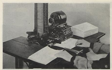
ADDRESSOGRAPH MODEL "F-2" OPERATION No. 2 The operator removing the addressed envelope and inserting another by hand. In this type of machine the smooth, easy operation of Warren's Standard Booklet Envelopes is particularly noticeable
