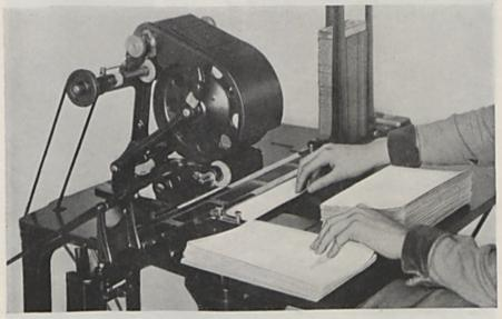
ELLIOTT ELECTRIC DRIVE ADDRESSER Another type of addressing machine fed by hand but operated by electric drive. Here, again, the speed and smoothness of Warren's Standard Booklet Envelopes are most satisfactory to the operator
