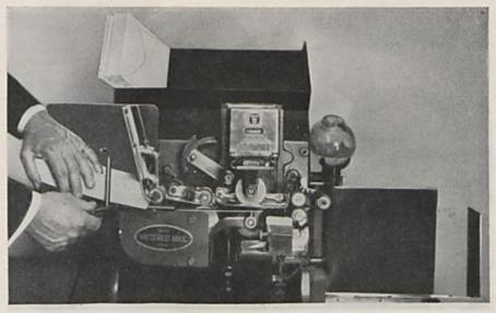
PITNEY-BOWES MODEL "B" OPERATION No. 2 The side guide is then set against the outer edge of the pile to hold the envelopes constantly at the proper position for smooth and even feeding into the machine
