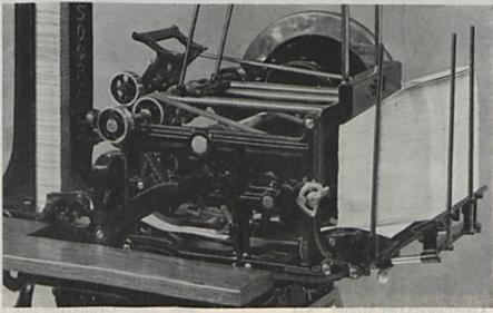
ADDRESSOGRAPH MODEL "A-1" OPERATION No. 2 The first envelope is shown in printing position in the lower left center of the illustration. Another envelope from the bottom of the feed pile is starting towards printing position
