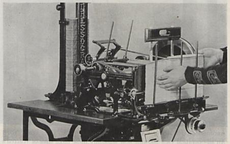
ADDRESSOGRAPH MODEL "A-1" OPERATION No. 1 The operator is stacking the envelopes flap up and adjusting the feed before starting the addressing machine. Note the large size of Warren's Standard Booklet Envelopes used in this demonstration
