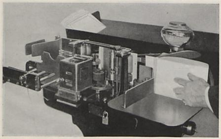
PITNEY-BOWES MODEL "A" OPERATION No. 3 The moistening and sealing having been completed in a single continuous operation, the envelope glides smoothly through pressure rolls into position for indicia printing as shown in the center of the illustration
