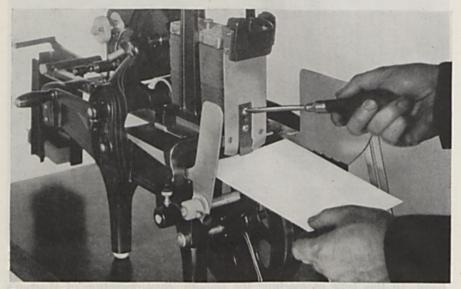
ELLIOTT MODEL "125" OPERATION No. 1 In this illustration the operator is setting the thickness gauge to correspond with the exact *thickness* of the envelope to be used. Note that the envelope is inserted flap down
