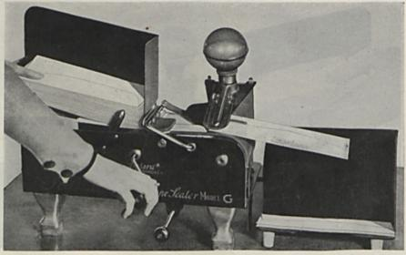
STANDARD MODEL "G" OPERATION No. 4 The conclusion of the sealing process. One sealed envelope is about to leave the machine as the corner of the following envelope rises evenly over the "ploughshare." The flap operates as smoothly at the end as at the start of the sealing process
