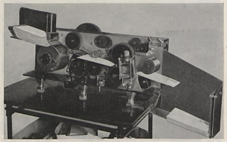
STANDARD POSTAL PERMIT PRINTER AND SEALER OPERATION No. 4 An all-process view showing how rapidly and easily Warren's Standard Booklet Envelopes pass through this permit printer and sealer. The sealed envelope at the right is about to leave the pressure rolls
