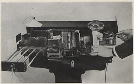
PITNEY-BOWES MODEL "A" OPERATION No. 1 In this vertical feed machine, the envelope is sealed *before* the indicia is printed. After opening the flaps, the operator is setting the feeding and sealing device to correct position
