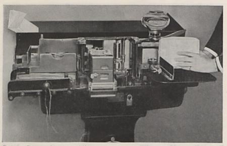
PITNEY-BOWES MODEL "A" OPERATION No. 2 The envelope is now in feeding position. The flap, well opened, passes smoothly over the feeding guide directly in front of the water container, is moistened and closed, passing on to pressure rolls
