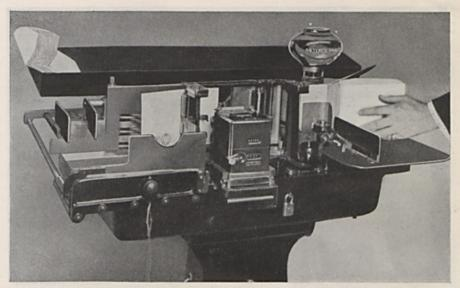
PITNEY-BOWES MODEL "A" OPERATION No. 4 Printed with the indicia stamp, the already sealed envelope is smoothly delivered to the jogger while the next envelope is being sealed
