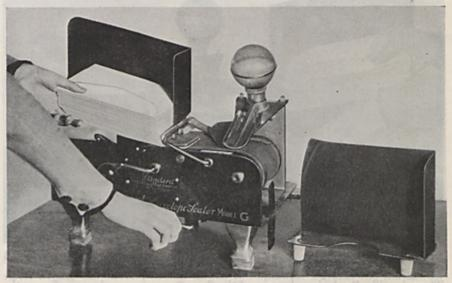
STANDARD MODEL "G" OPERATION No. 1 The envelopes are placed flap up in the feeding device and the operator sets the back guide and moistening device in correct position
