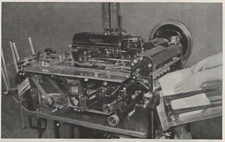
ADDRESSOGRAPH MODEL "A-4" OPERATION No. 1 In this type of Addressograph the operator is adjusting the stack of envelopes before starting the machine. The envelope at the extreme left of the pile will be carried to printing position
