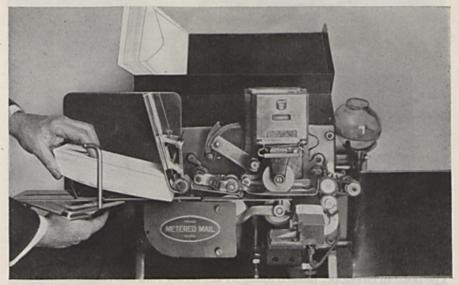
PITNEY-BOWES MODEL "B" OPERATION No. 1 The envelopes are placed flap down. With the right hand the back guide is set at the correct feeding angle so that the bottom envelope will slide easily into the machine
