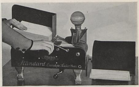
STANDARD MODEL "G" OPERATION No. 2 The operator feeds the envelopes into the sealer by turning the crank. As the envelope approaches the moistener, the flap is easily raised and rides smoothly up and over the "ploughshare"
