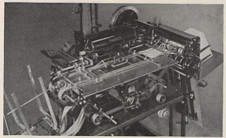
ADDRESSOGRAPH MODEL "A-4" OPERATION No. 2 This view shows the envelope in the pneumatic feed and approaching printing position. The smoothness of operation here is especially gratifying to the operator of the Addressograph
