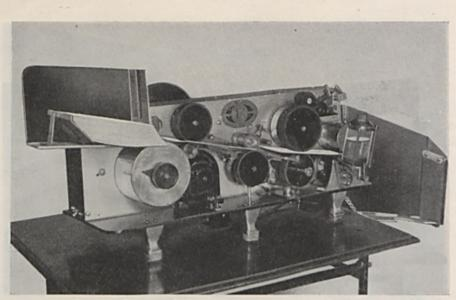
STANDARD POSTAL PERMIT PRINTER AND SEALER OPERATION No. 3 This view shows the first envelope passing through the printing rolls as the second envelope smoothly approaches printing position. The first envelope is approaching the sealing device
