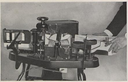
PITNEY-BOWES MODEL "AM" OPERATION No. 5 View showing the complete sealing process of Warren's Standard Booklet Envelopes in the MAIL-O-METER. Notice how easily and effectively the correctly designed flap keeps contact as it passes over the moistener after which the flap is sealed by the pressure rolls
