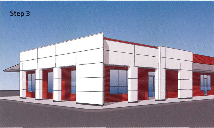
To minimize business interruption and construction costs, new architectural elements were installed around the building envelope.
