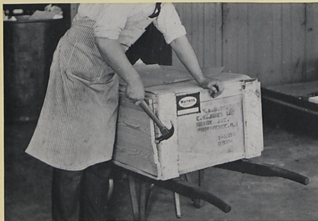
To avoid dust and dirt in unpacking paper, first place case right side up. Remove nails from top boards as shown in upper picture. Then loosen side boards as shown in lower picture. For next steps see page 6
