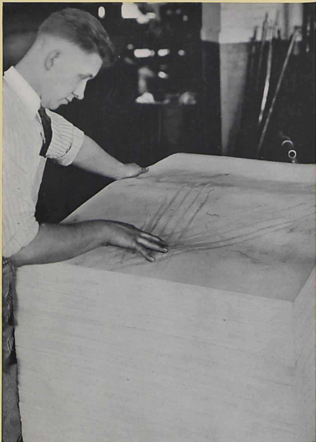
ANY sheet of paper that lays around any printing plant for twenty-four hours will give plenty of evidence of the fact that the air is constantly full of particles of dust and dirt. This pile of paper had so much dust on it that streaks are left where the fingers were drawn over the top
