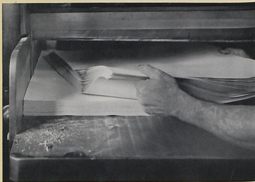
THESE pictures show how particles broken off from the edges in cutting and lint accumulate on cutter. Unless this dust is wiped away, much of it is picked up by edges of paper as it is fanned and pushed against the side plate
