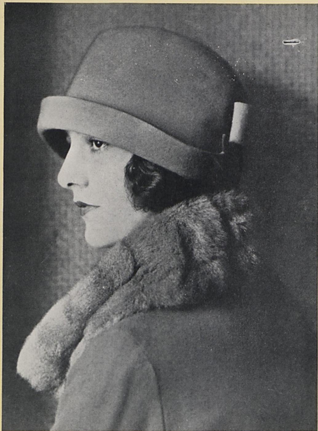
THIS is a halftone reproduction of a printed result from a plate on which a hard substance (a brush bristle in this instance) had fallen—see upper right-hand corner. The hard substance coming between the plate and the paper holds the paper from the plate, making the white circle around it. See magnified section at top of opposite page
