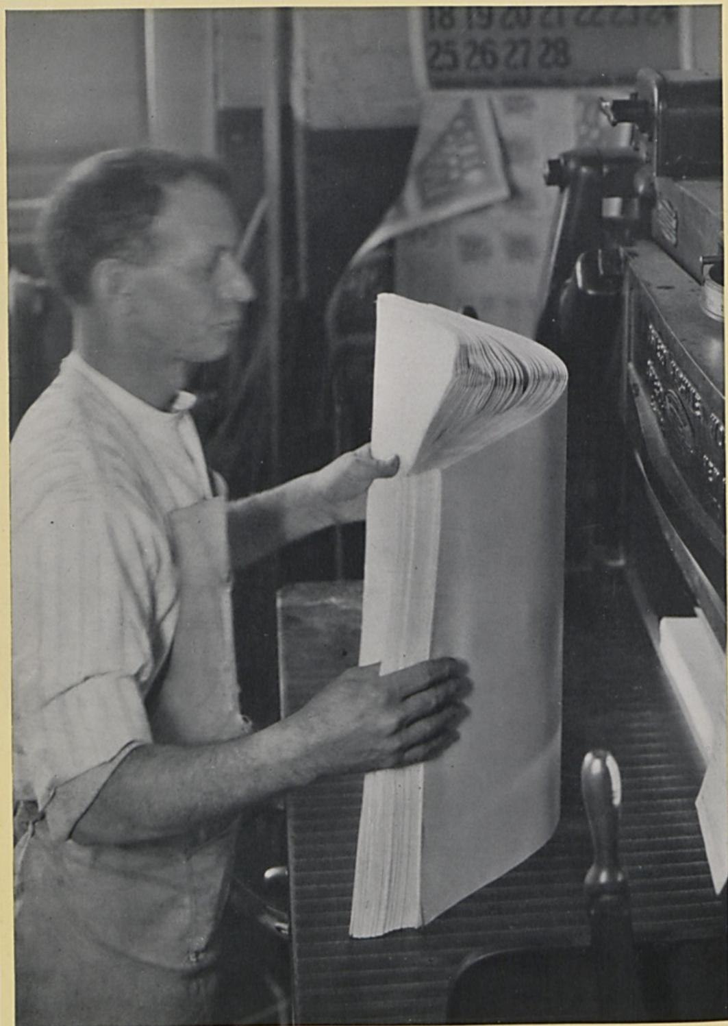
If dust is gathered up on the cutter as shown on page 10, it sifts down between sheets of paper when the lift is winded and jogged as shown here. If dust is found on sides of lift, it should be shaken off before the jogging operation
