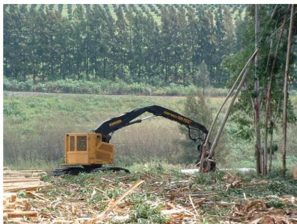
**Photo 11a:** Tracked single stem harvester (CTL system)
