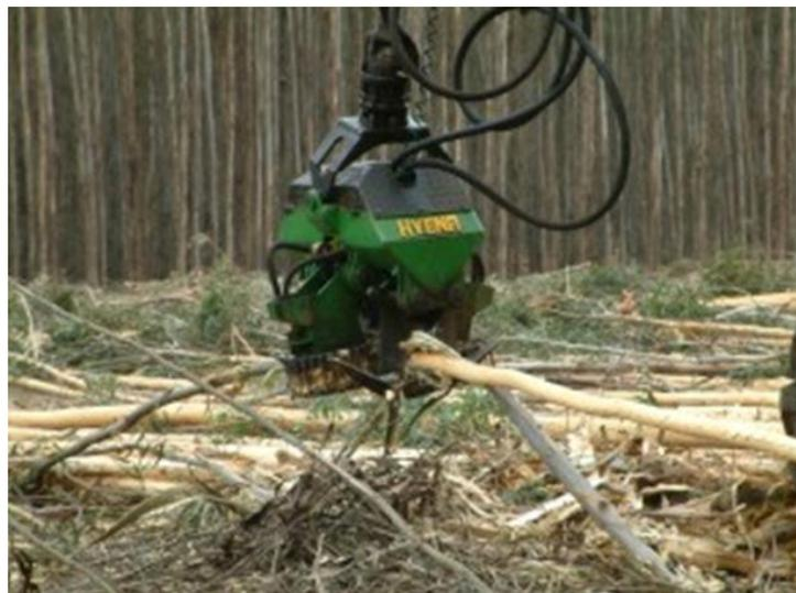
**Photo 9:** Locally designed debarking head<sup>3</sup>
