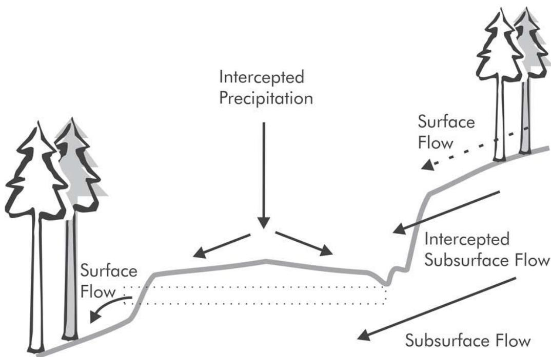
**Figure 8:** The effect of forest roads on surface and subsurface flow.<sup>10</sup>
