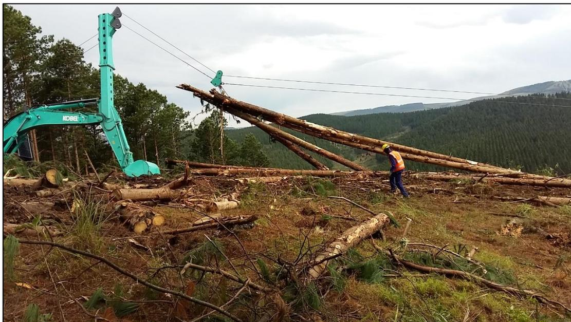
The use of shovel yarders is increasing as opposed to traditional high-leads and skylines. Apart from being safer, it's quick to set up and therefore increases productivity.
