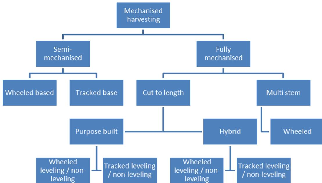
**Figure 7:** Classification of mechanised harvesting systems
