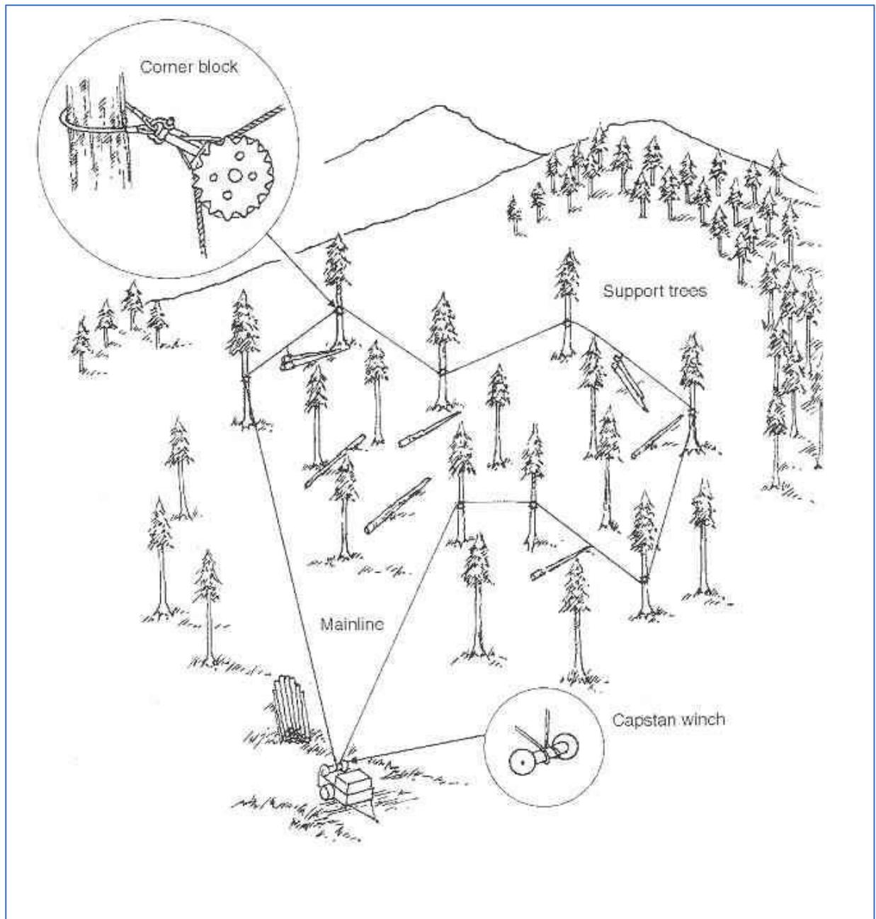
Figure 7: Monocable system.<sup>8</sup>
