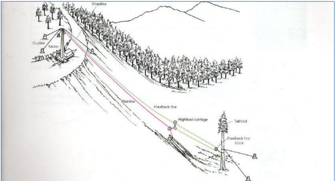
**Figure 4:** High-lead system with a carriage as used in South Africa.<sup>8</sup>
