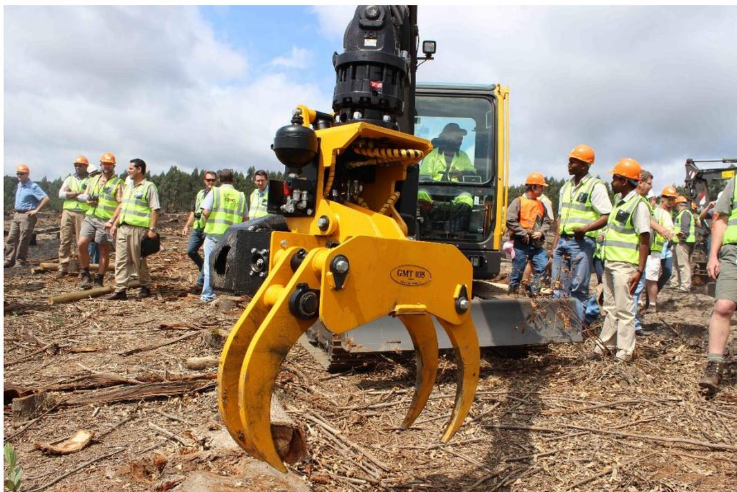
**Photo 15:** This felling grapple weighs just 225 kg and can be mounted on a truck-mounted crane, a three-wheeler, or a small excavator. It can cut standing trees up to 350 mm diameter.<sup>8</sup>
