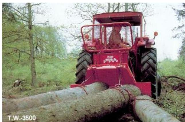
**Photo 2a:** Tractor with winch ([www.logloader.com](http://www.logloader.com))
