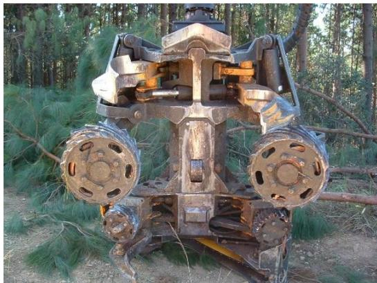
**Photo 13 (left):** Shear type felling head<sup>7</sup>
