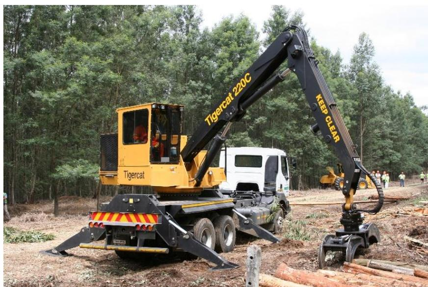
**Photo 7:** Truck-mounted knuckle boom loader.<sup>6</sup>
