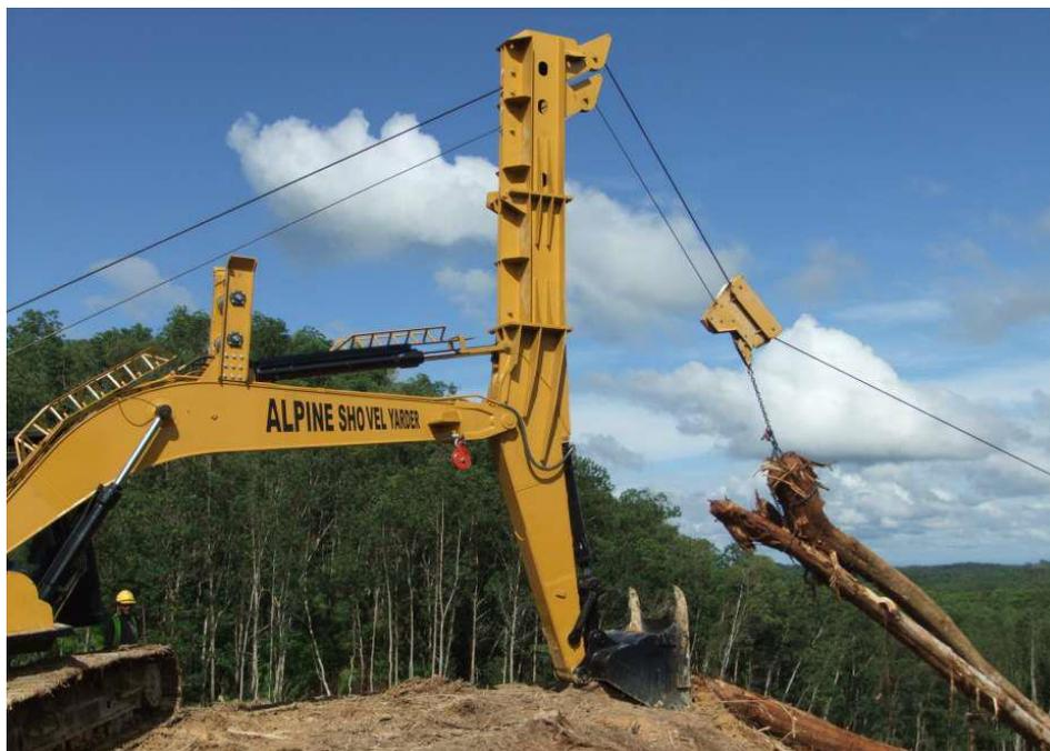
**Photo 5:** High power double drum shovel yarder with extended tower.<sup>9</sup>
